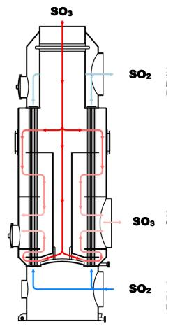
The patented SF™ Exchanger eliminates the need for sacrificial gas exchangers offered by some contractors.
